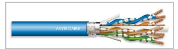
Level twist pair cable suitable for digital communication, Used in Building integrated wiring system, for the working area communication leads and connecting rack between the handover, Meet the 100 MHz in the data communication. coloring According to the ANSI/TIA/EIA-568-B color coding standard.
